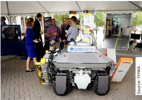
The RABIT™ bridge deck assessment tool on display at FHWA Research Day.
