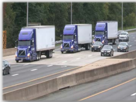
A three-truck platoon using CACC technology.
