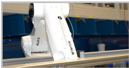
The lab's robotic arm can be used to visually record water passing over a scale model.
