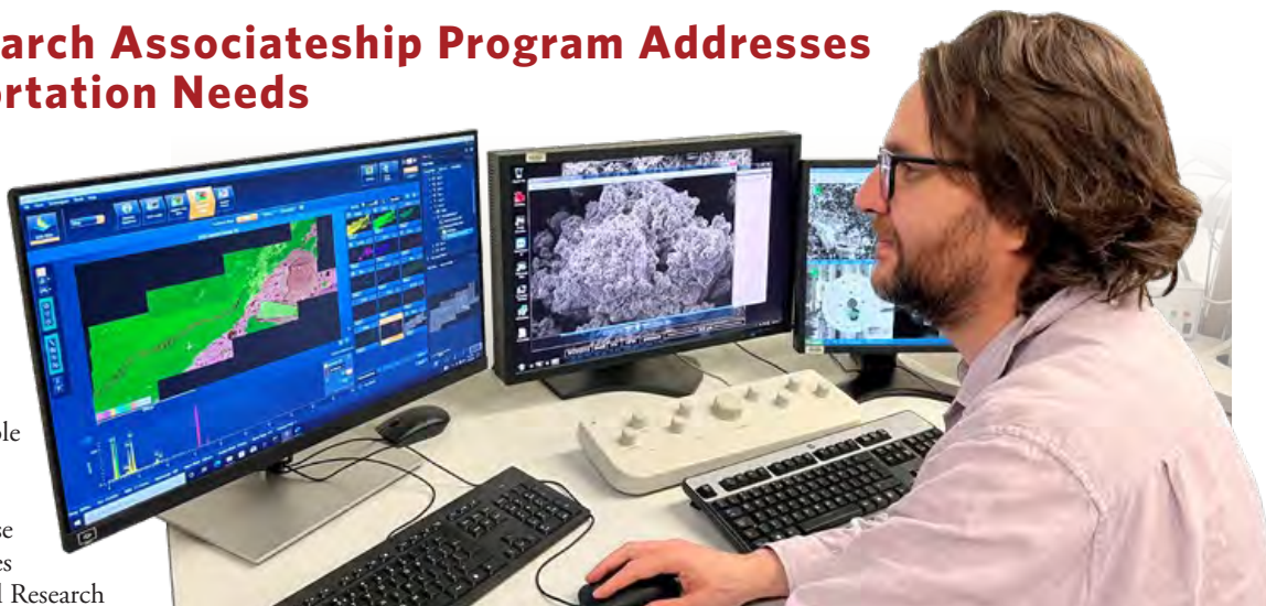
Dr. Campos uses a scanning electron microscope to examine a concrete core from a bridge. Source: FHWA.
