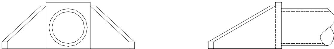
**Figure 23. Mitered 30-degree wingwall configuration.**
