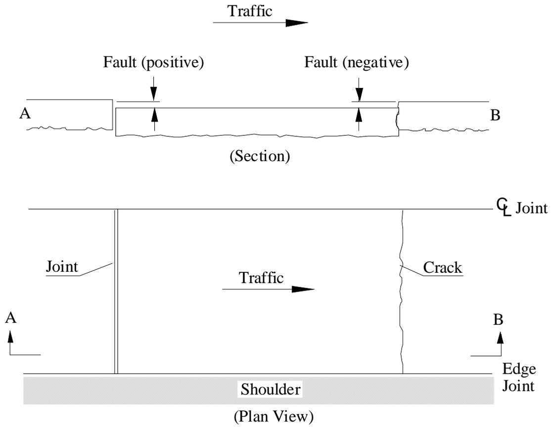
Figure 3. Faulting of transverse joints and cracks.
