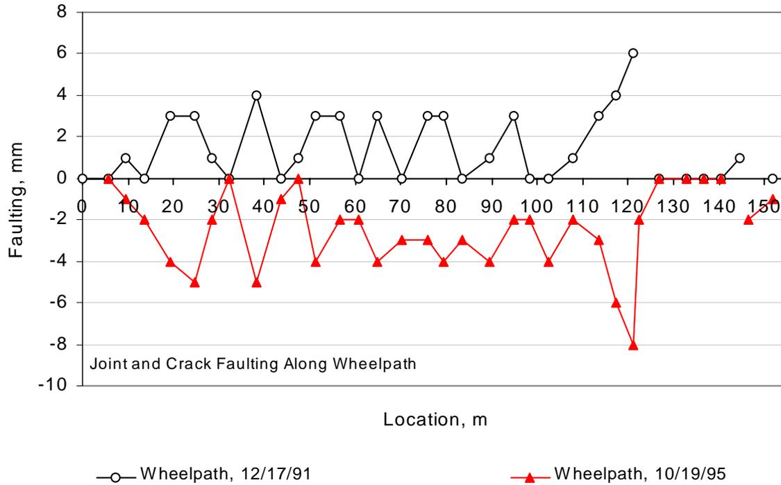
Figure 4. Example of the negative mirror image faulting (GPS-3 section 067458).
