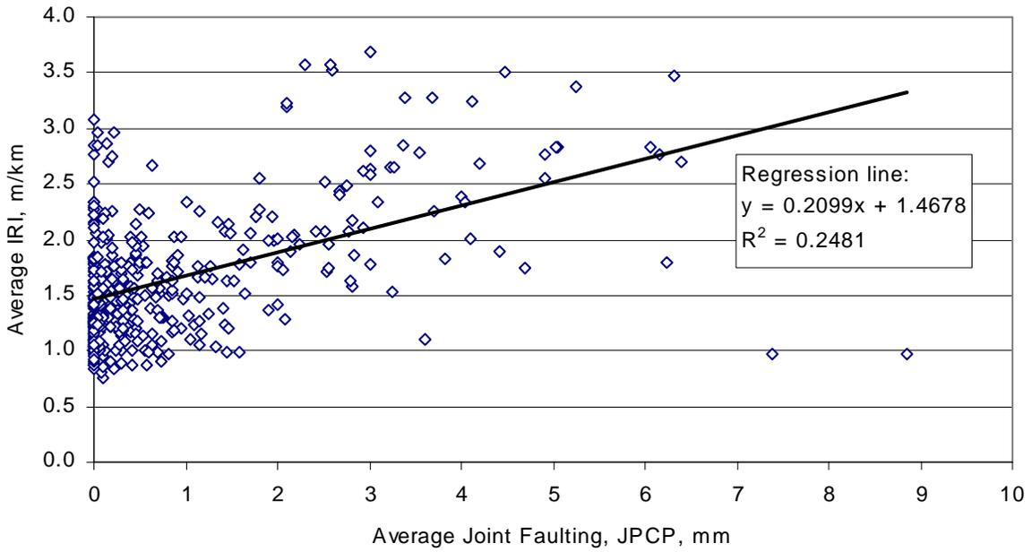
Figure 17. Average faulting versus average IRI for JPCP sections (initial IRI not considered).
