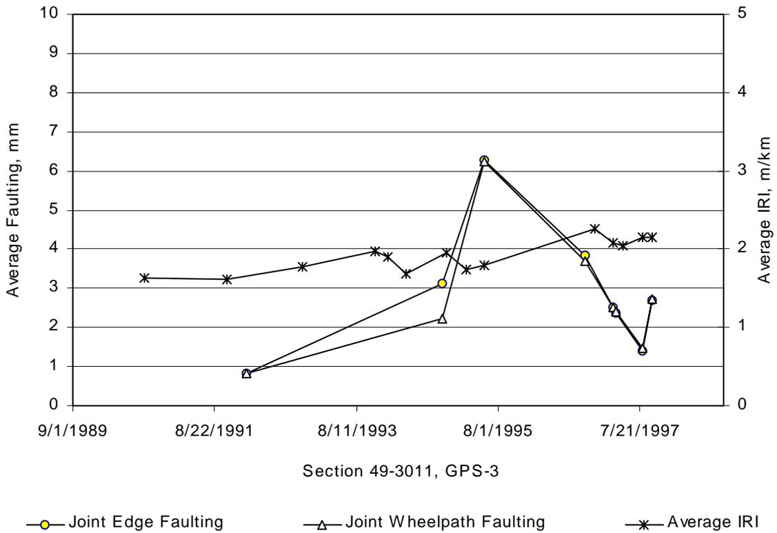
Figure 16. Example of "poor" correlation between faulting and IRI trends.
