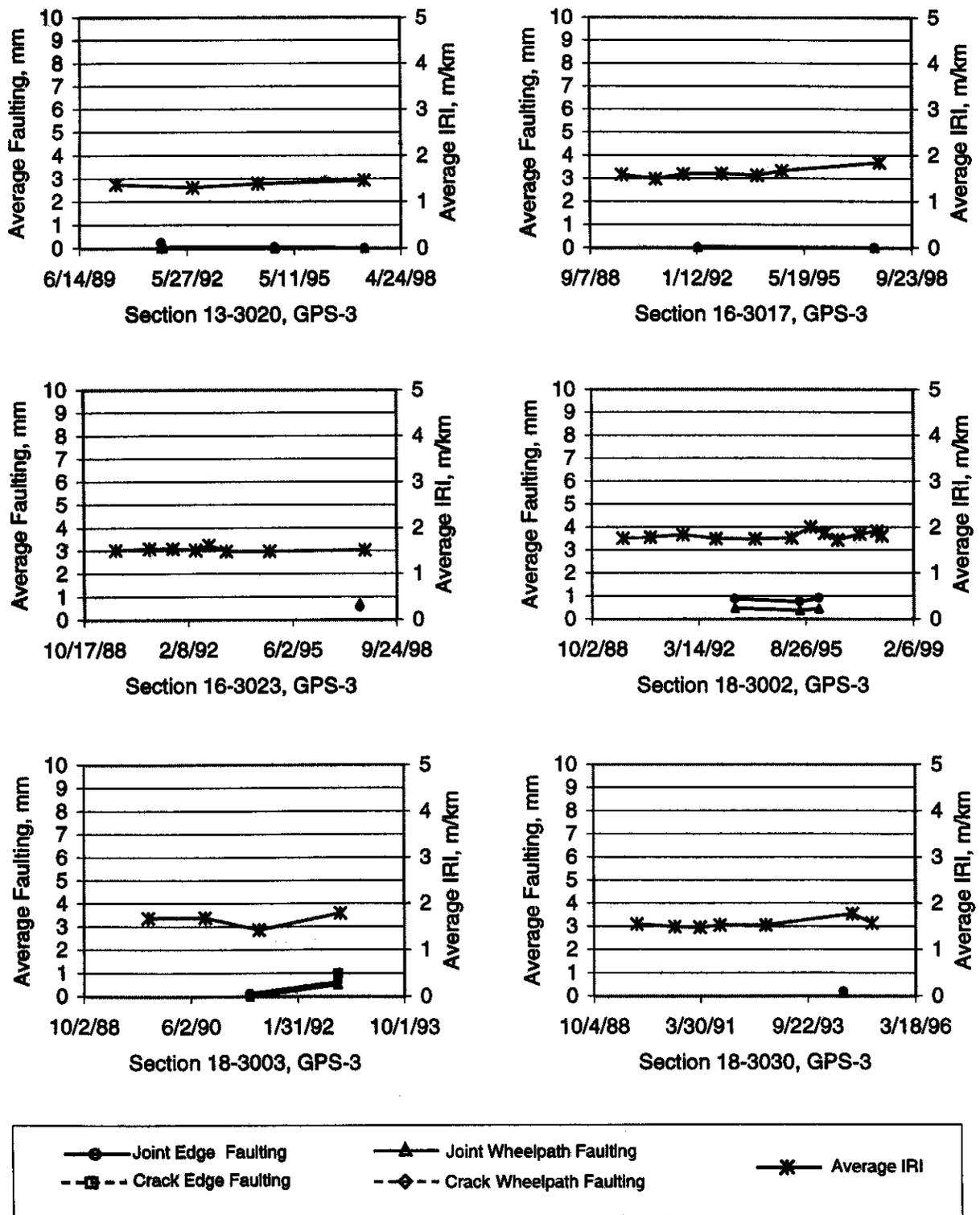
Figure 33. Time series plots for GPS-3 sections 133020, 163017, 163023, 183002, 183003, and 183030.
