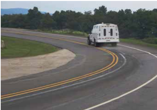
FHWA's Highway Friction Tester, shown here, can assess pavement friction continuously through intersections and around curves.
