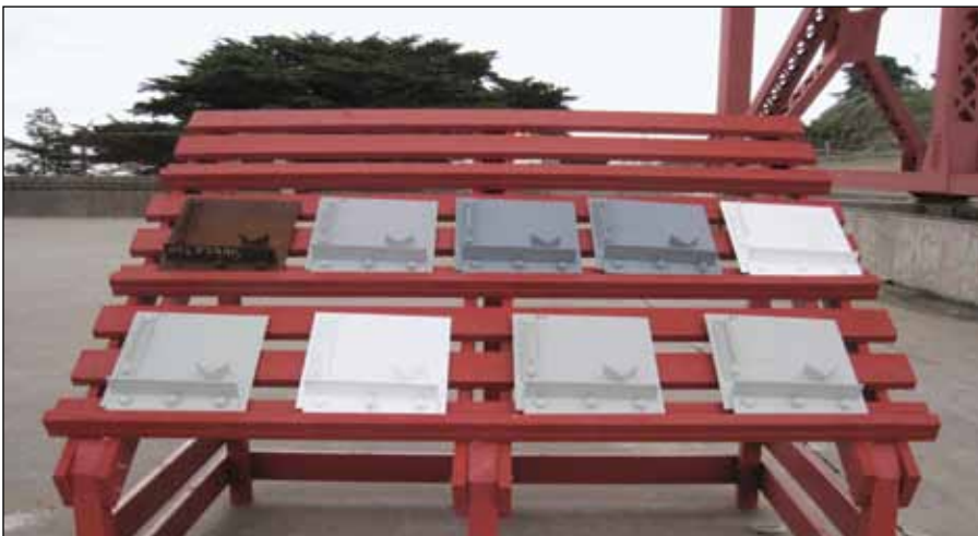
These coated type II panels were deployed at the Golden Gate Bridge.
