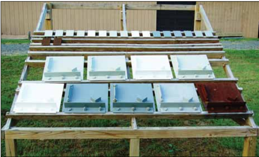
Type I (top row) and II (bottom rows) panels displaying a variety of coating types were arrayed on this rack for natural weathering testing at TFHRC in McLean, VA.
