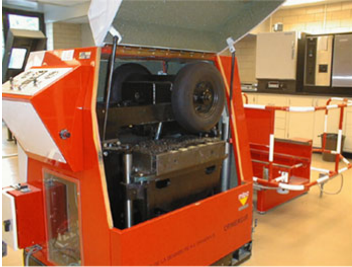
Figure 17. French Pavement Rutting Tester.
