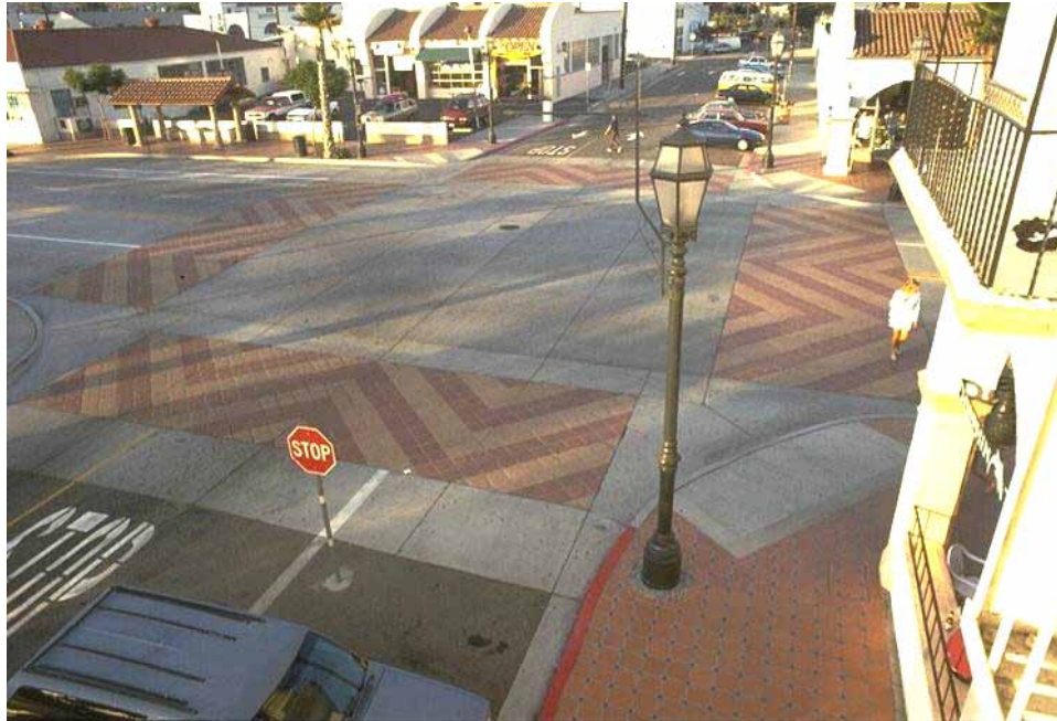
Figure 20-18. Photo. Pavement treatments can be applied to the entire traffic-calmed area or limited to specific street uses.
