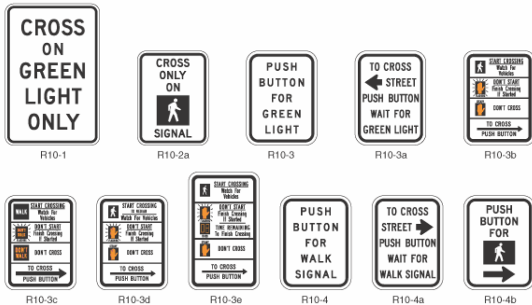
Figure 10-2. Photo. Pedestrian crossing signs. Source: MUTCD (1)
