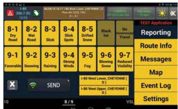
**Connected vehicle-enabled weather responsive traffic management (WRTM) combines traditional traffic management with connected vehicle (CV) technologies.**
