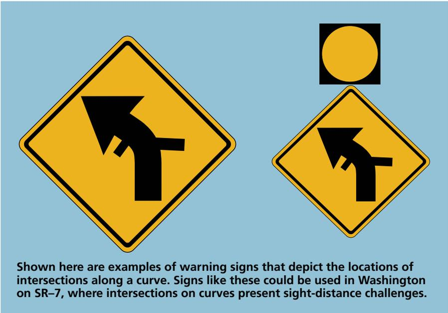
In addition, the RSA team suggested some short-range actions for other RSA sites on the SR-7 corridor to improve motorcycle safety, such as installing intersection warning signs that indicate an upcoming intersection, installing reflective post-mounted delineators that are evenly spaced throughout both sides of curves, applying wider edge lines and center lines, and installing shoulder rumble strips.
