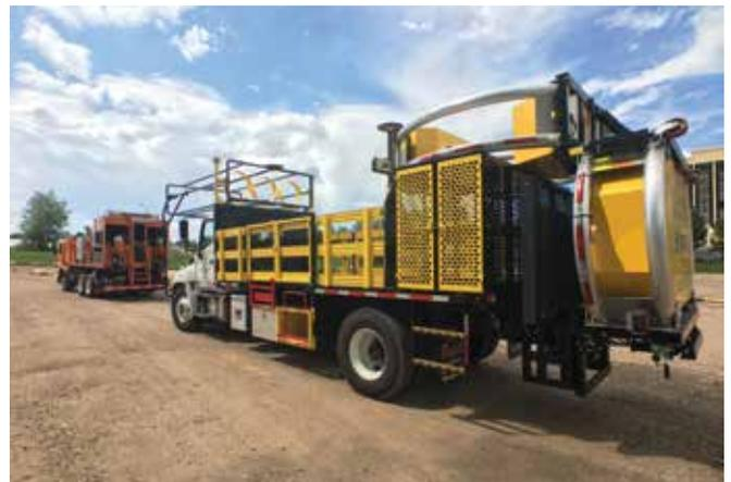
**Colorado's Autonomous Impact Protection Vehicle increases work zone safety by removing the driver from a vehicle designed to provide a buffer between traffic and roadway workers.**
