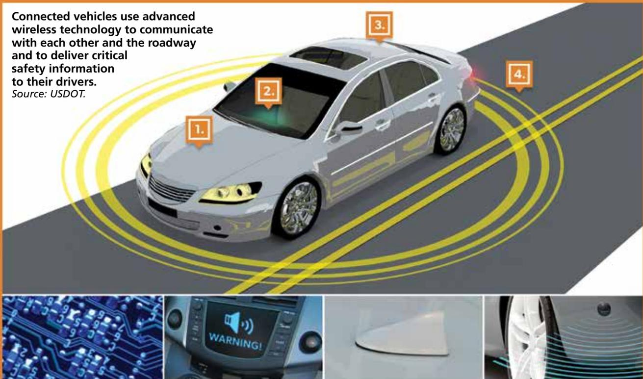
1. An under-the-hood box (a processor with memory) collects and transmits data between the vehicle's onboard equipment (OBE) and between OBE on nearby connected vehicles and safety devices along the roadside.
