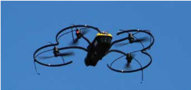
**Highway agencies use unmanned aerial systems—or drones—like this one for surveying, inspections, and monitoring.**
