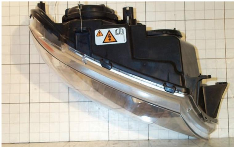
**Figure 37. Photo. High intensity discharge 2 plan view.**
