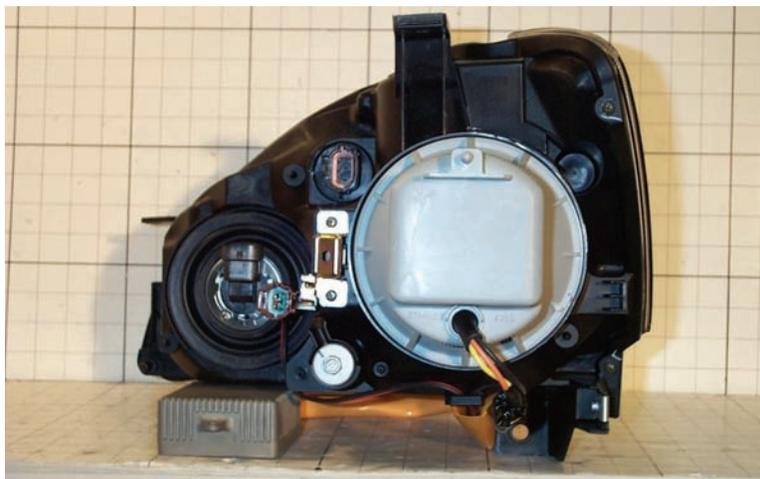
**Figure 43. Photo. High intensity discharge 3 rear view.**
