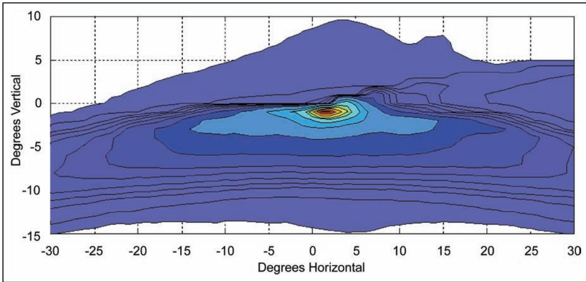
**Figure 34. Graph. High intensity discharge low beam 1 isocandela plot (right headlamp).**
