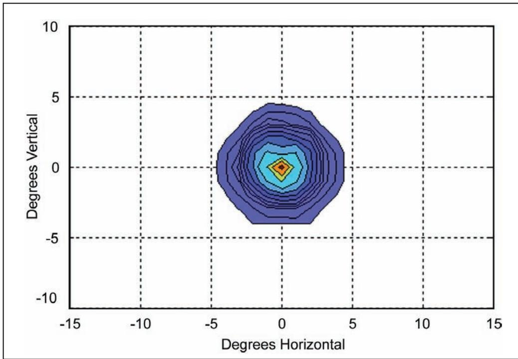
**Figure 58. Graph. UV-A isoWatt plot of radiant intensity.**
