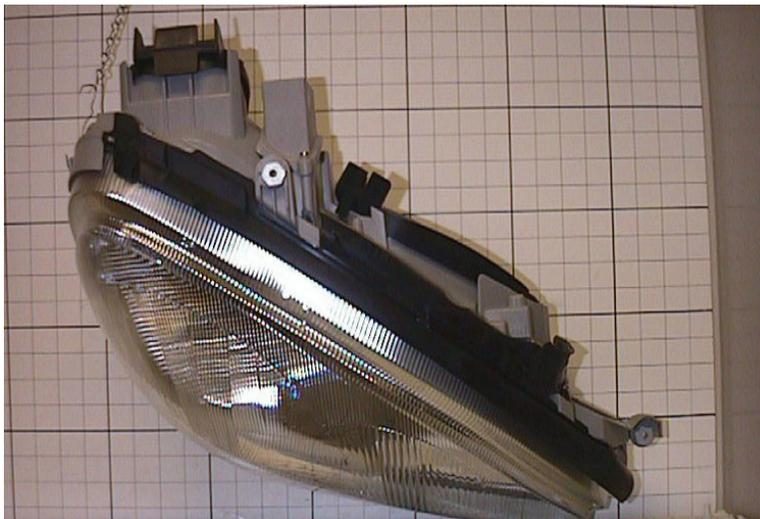
**Figure 25. Photo. High intensity discharge plan view.**
