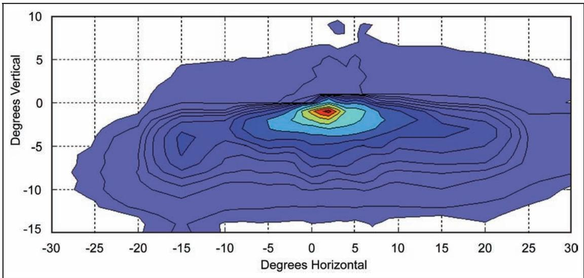
**Figure 20. Graph. Halogen low beam low profile isocandela plot (right headlamp).**
