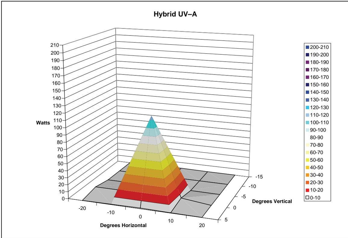
**Figure 51. Graph. Hybrid UV-A radiant intensity.**
