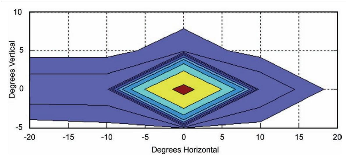
**Figure 52. Graph. Hybrid UV-A isoWatt plot of radiant intensity.**
