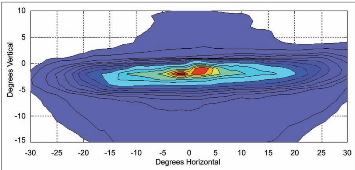
**Figure 39. Graph. High intensity discharge low beam 2 isocandela plot (right headlamp).**
