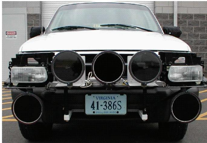
Upper row of headlamps used for three UV-A configurations.
