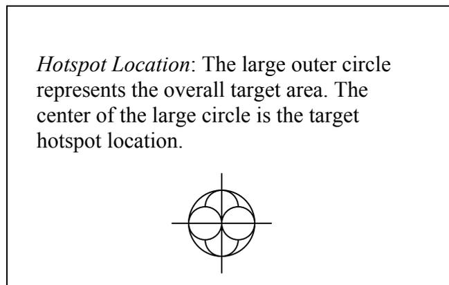
To determine if the hotspot is in the correct location, you will need to use the International Light, Inc., IL1400A Radiometer/Photometer to measure the area of greatest intensity. There are two sensors for the photometer; the sensor for the visible light is marked with a “REG” label, and the sensor for the UV light is marked with a “UV–A” label. For UV–A light, use the photometer sensor marked “UV–A.”
