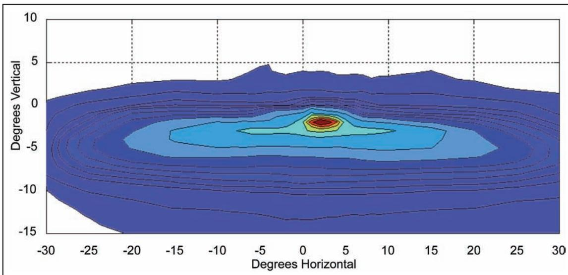
**Figure 28. Graph. Companion headlamp to NIR 2 and FIR isocandela plot (right headlamp).**
