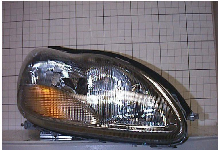
**Figure 23. Photo. High intensity discharge front view.**
