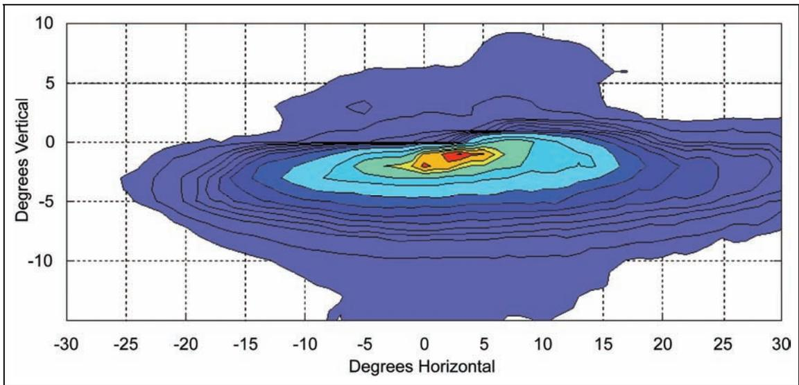
**Figure 44. Graph. High intensity discharge low beam 3 isocandela plot (right headlamp).**
