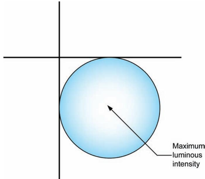
**Figure 9. Diagram. Hotspot aiming for mechanically aimed lamps.**
