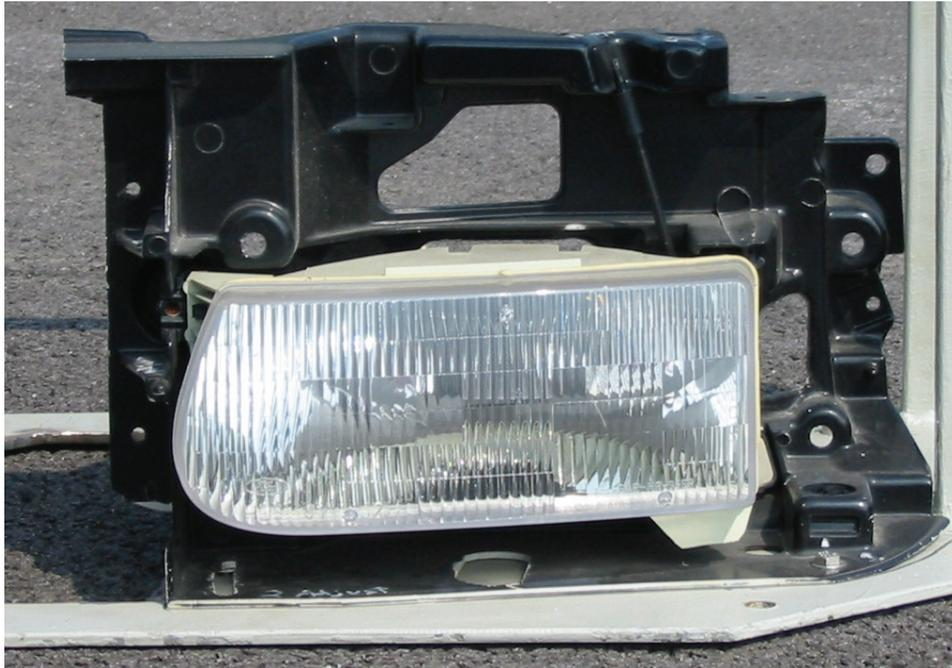
**Figure 17. Photo. Halogen low beam front view.**
