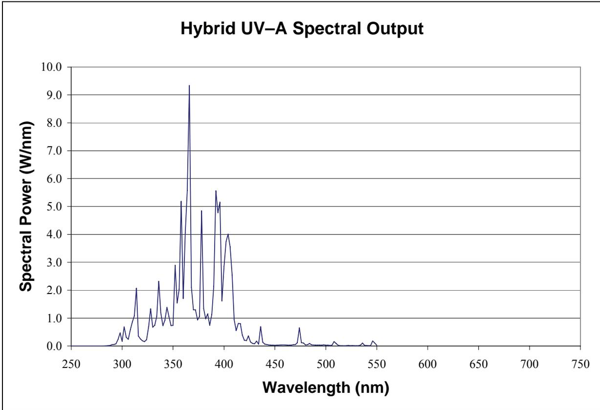
Figure 46. Line graph. Spectral power distribution of the hybrid UV-A source.
