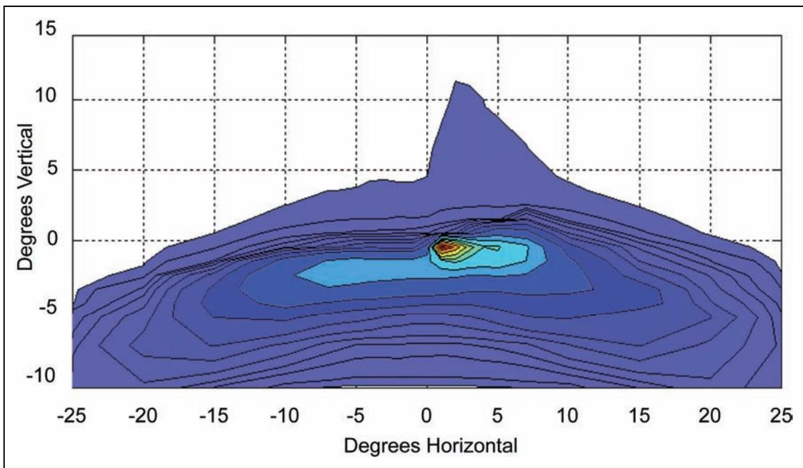
**Figure 27. Graph. High intensity discharge low beam isocandela plot (right headlamp).**
