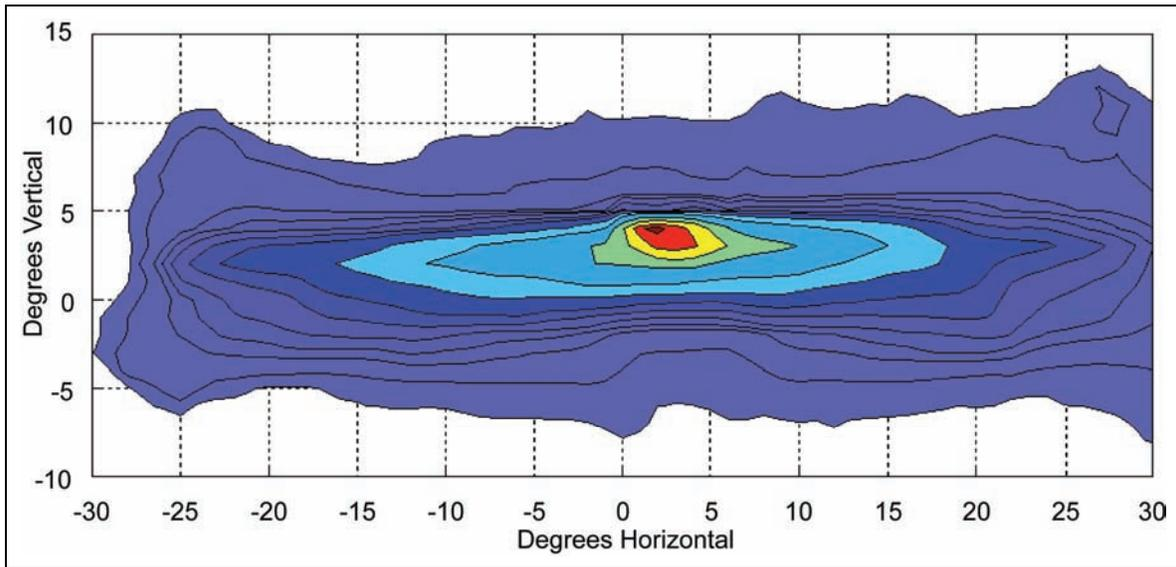
**Figure 29. Graph. Companion headlamp to NIR 1 isocandela plot (right headlamp).**
