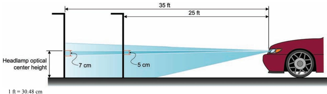
**Figure 6. Diagram. Comparison of vertical reference point for 25-ft and 35-ft headlamp alignment distances.**
