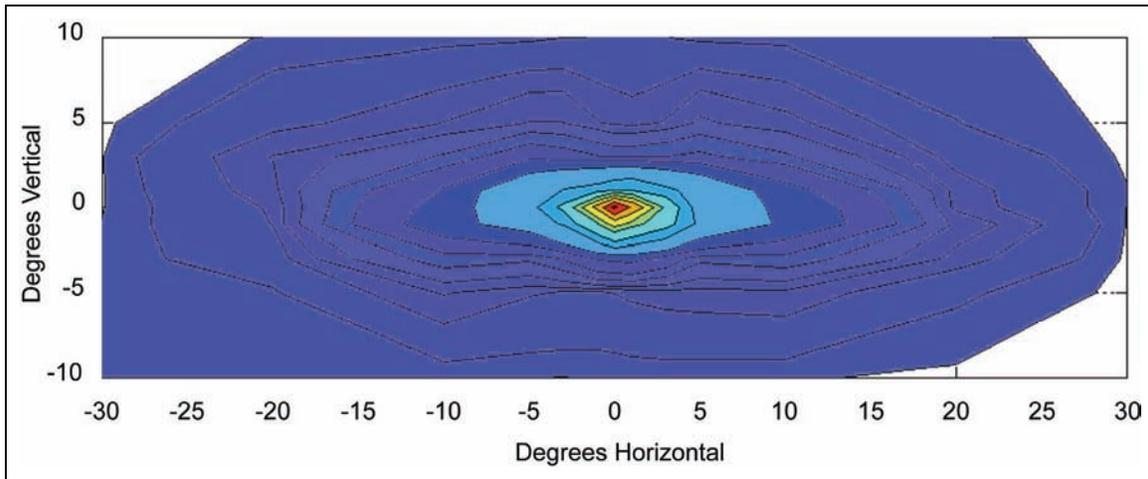
**Figure 21. Graph. Halogen high beam isocandela plot (right headlamp).**
