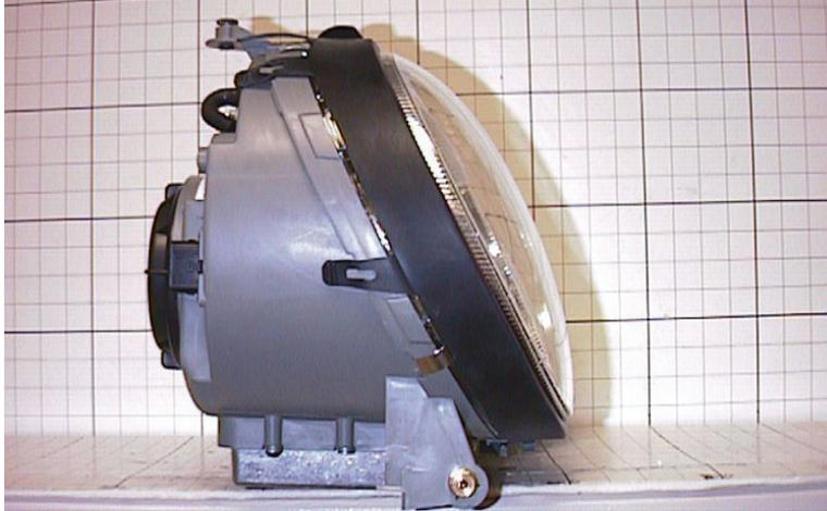
**Figure 31. Photo. High intensity discharge 1 side view.**
