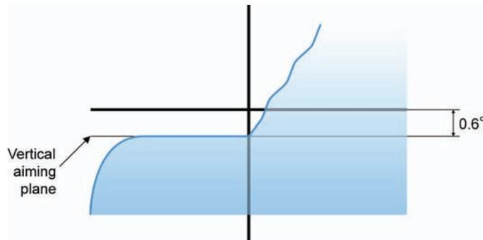
**Figure 7. Diagram. VOL aiming.**
