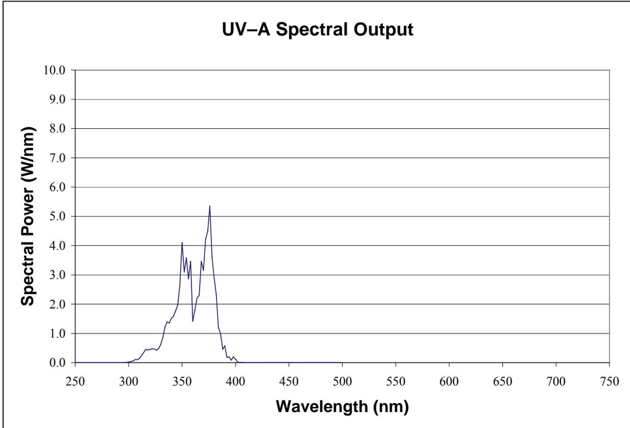
Figure 45. Line graph. Spectral power distribution of the UV-A source.
