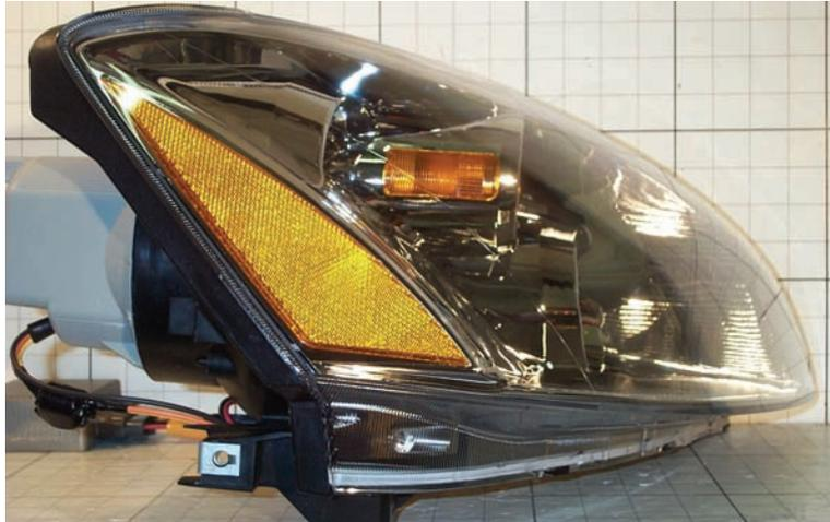
**Figure 41. Photo. High intensity discharge 3 side view.**
