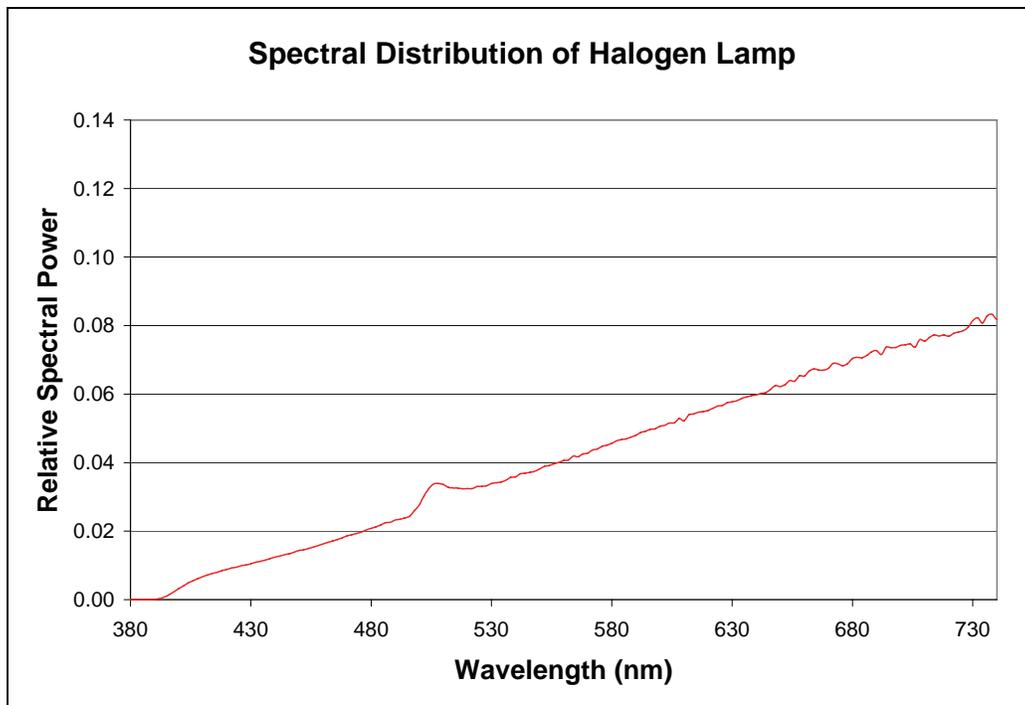
**Figure 12. Line graph. Visible light spectral power distribution of halogen lamp ranging from 380 nm to 730 nm.**
