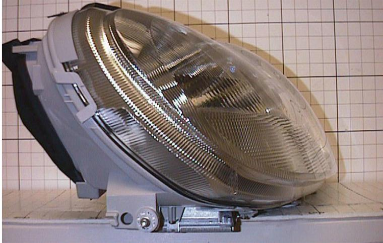
**Figure 24. Photo. High intensity discharge side view.**
