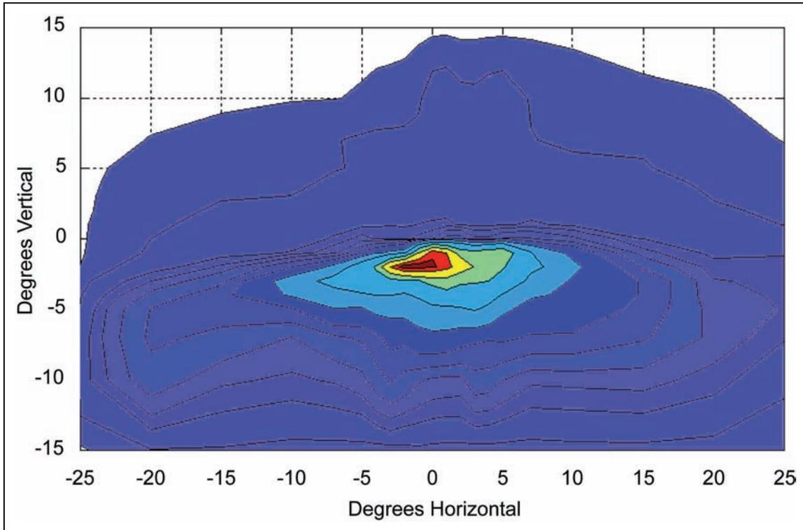
**Figure 22. Graph. High output halogen low beam isocandela plot (right headlamp).**
