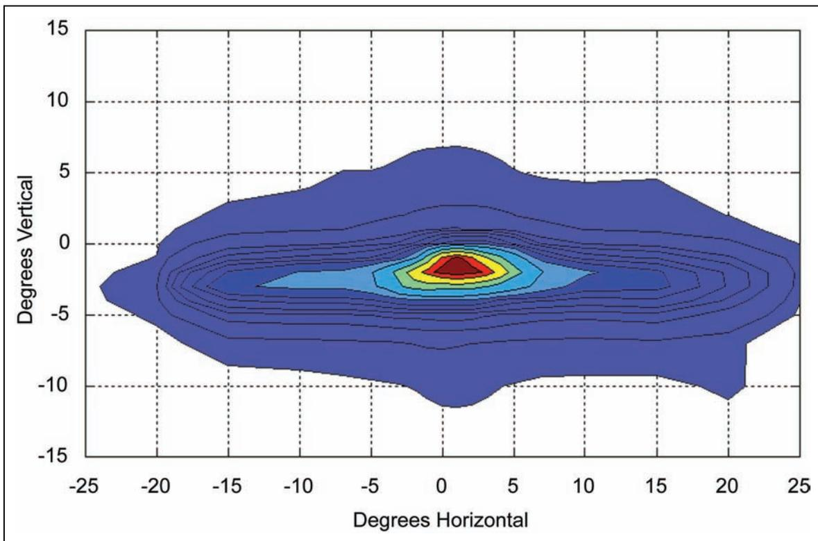
**Figure 18. Graph. Halogen low beam isocandela plot (right headlamp).**
