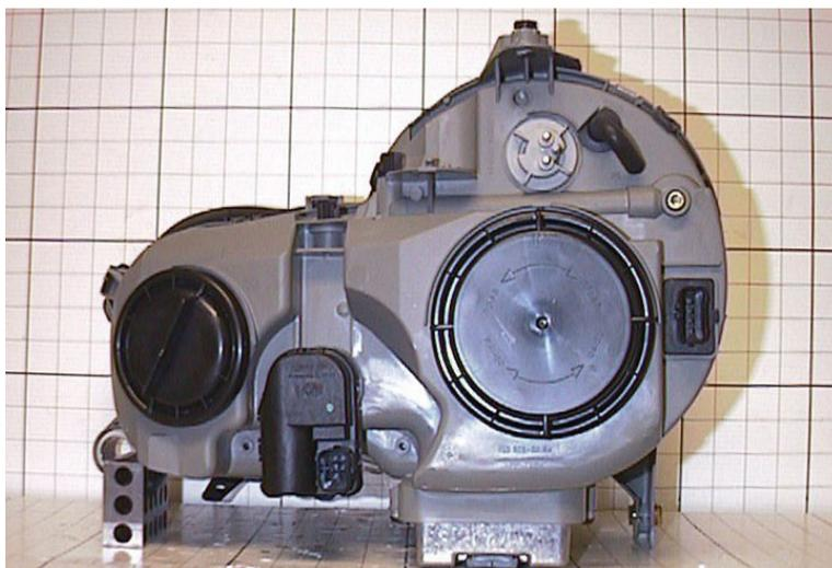
**Figure 33. Photo. High intensity discharge 1 rear view.**
