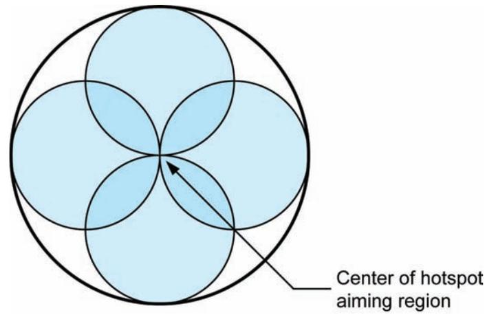
**Figure 11. Diagram. Hotspot aiming for UV-A lamps.**
