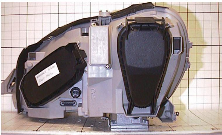
**Figure 26. Photo. High intensity discharge rear view.**
