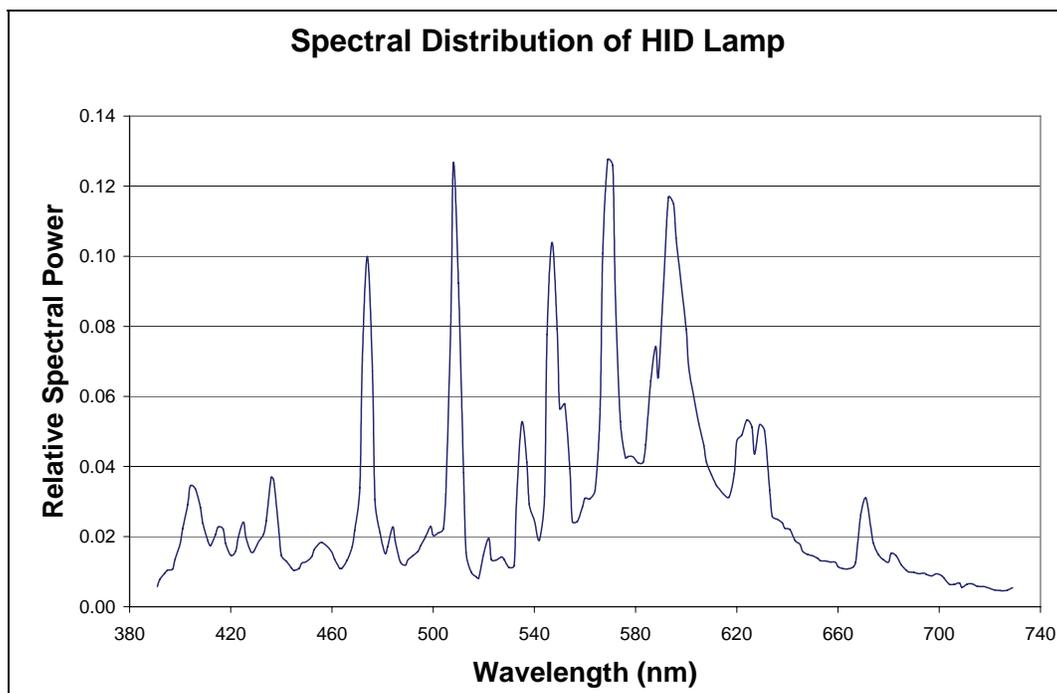
**Figure 13. Line graph. Spectral power distribution of HID lamp ranging from 380 nm to 740 nm.**
