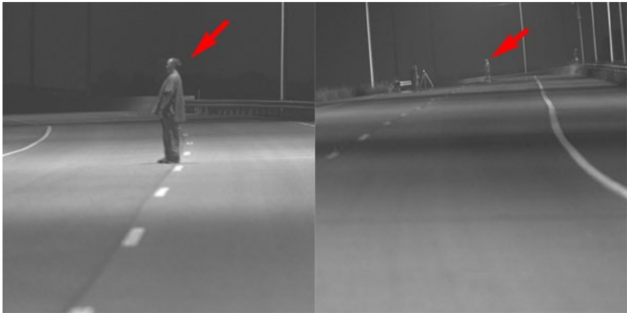
Figure 5. Photograph. Visual background for driver in a vehicle observing a pedestrian at 61 m (200 ft) and at 305 m (1,000 ft) from the pedestrian. Source: FHWA.
