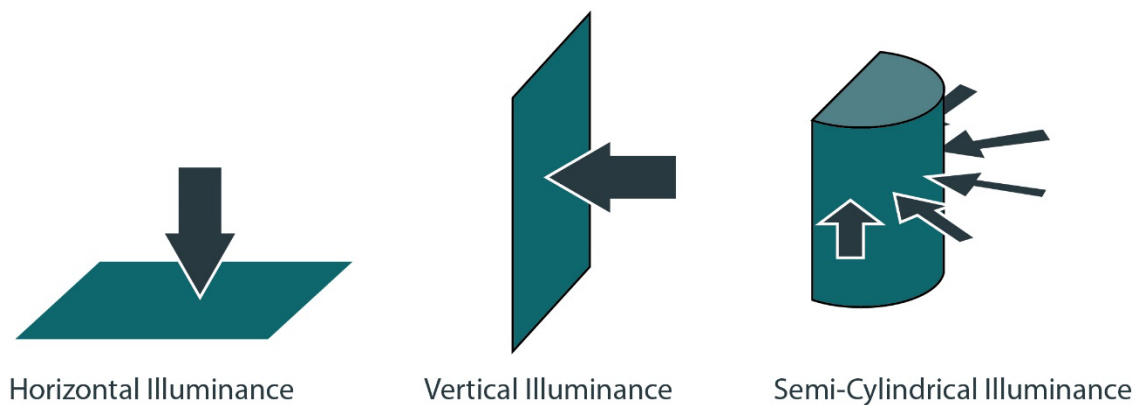
Figure 4. Graphic. Horizontal, vertical, and semi-cylindrical illuminance diagrams. Source: FHWA.
