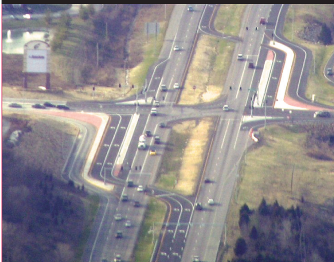
Figure 5. A partial DLT intersection in Fenton, MO.
