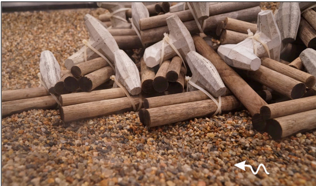
Figure 48. Photo. Log-dolos bundle from ELJ1 (upstream unit) turned upside down.
