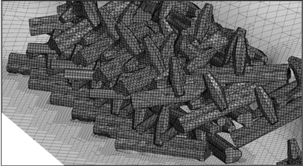
Figure 74. Graphic. Surface mesh representation of an ELJ unit.
