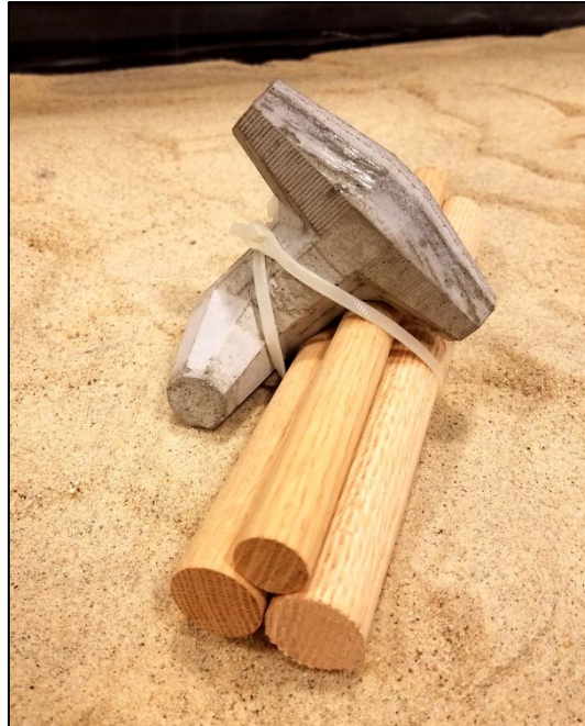
Figure 18. Photo. Fabricated log-dolos bundle (model scale 1:25).
