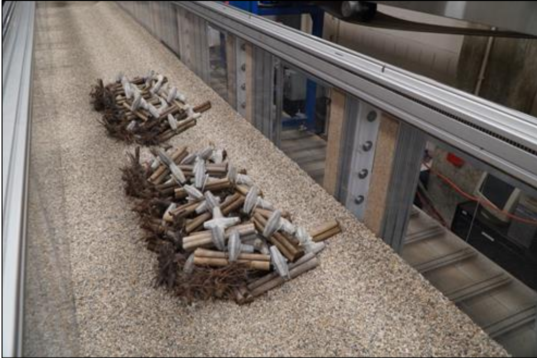
Figure 40. Photo. As-built ELJ installations on the erodible channel for run III-3.
