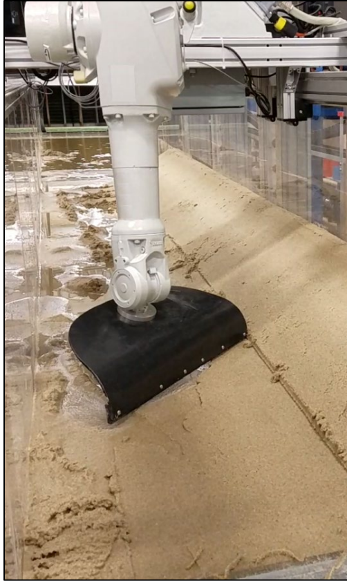
Figure 11. Photo. Robotic arm leveling the channel bed.
