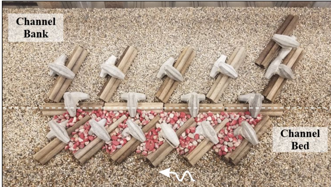
Figure 54. Photo. Plan view of one ELJ units showing installation of layer A filled with riprap for run III-7.
