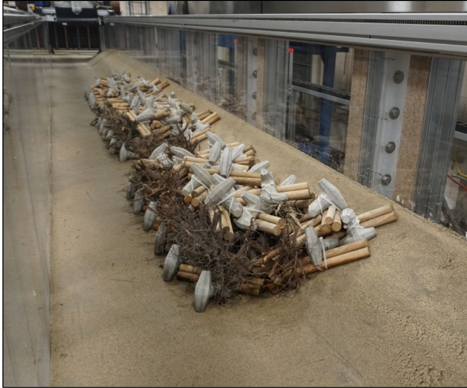
Figure 27. Photo. As-built ELJ installation for run I-3 with log-dolos bundles, rootwads, and key dolosse.
