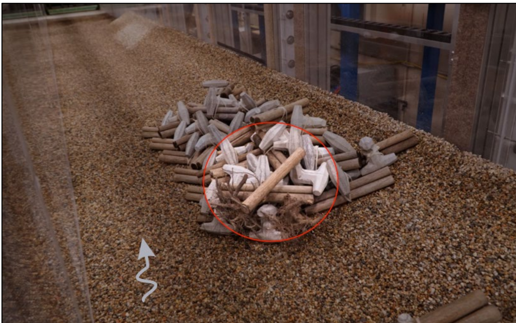
Figure 46. Photo. Fully submerged ELJ units in run III-4.
