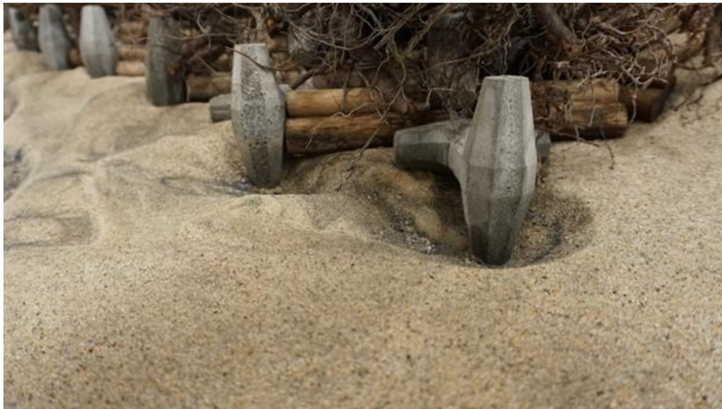
Figure 33. Photo. Local scour hole developed around the key dolosse in run I-2.
