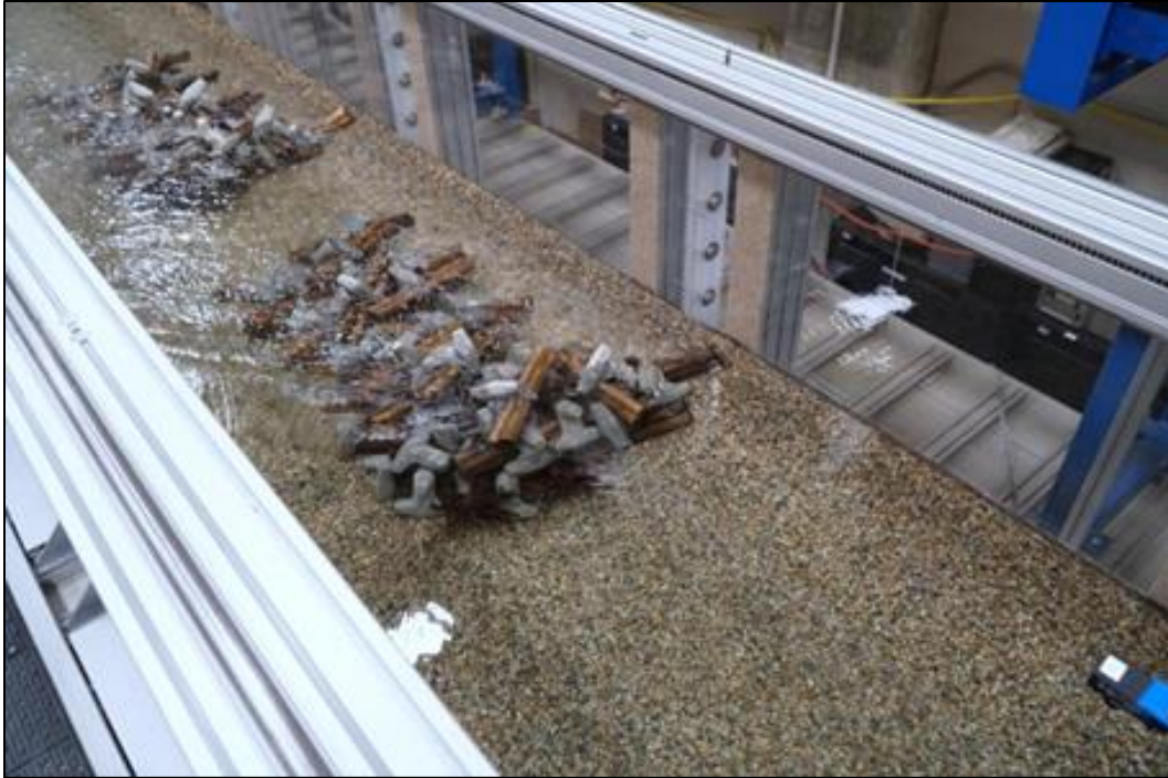
Figure 46. Photo. Fully submerged ELJ units in run III-4.
