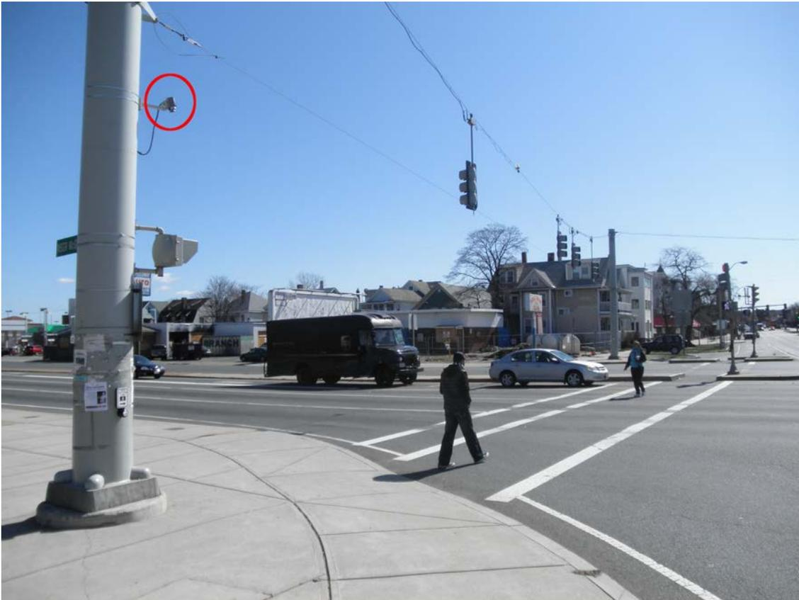
**Figure 2. Photo. Stereo camera mounted on a pole above a pedestrian walk signal.**
