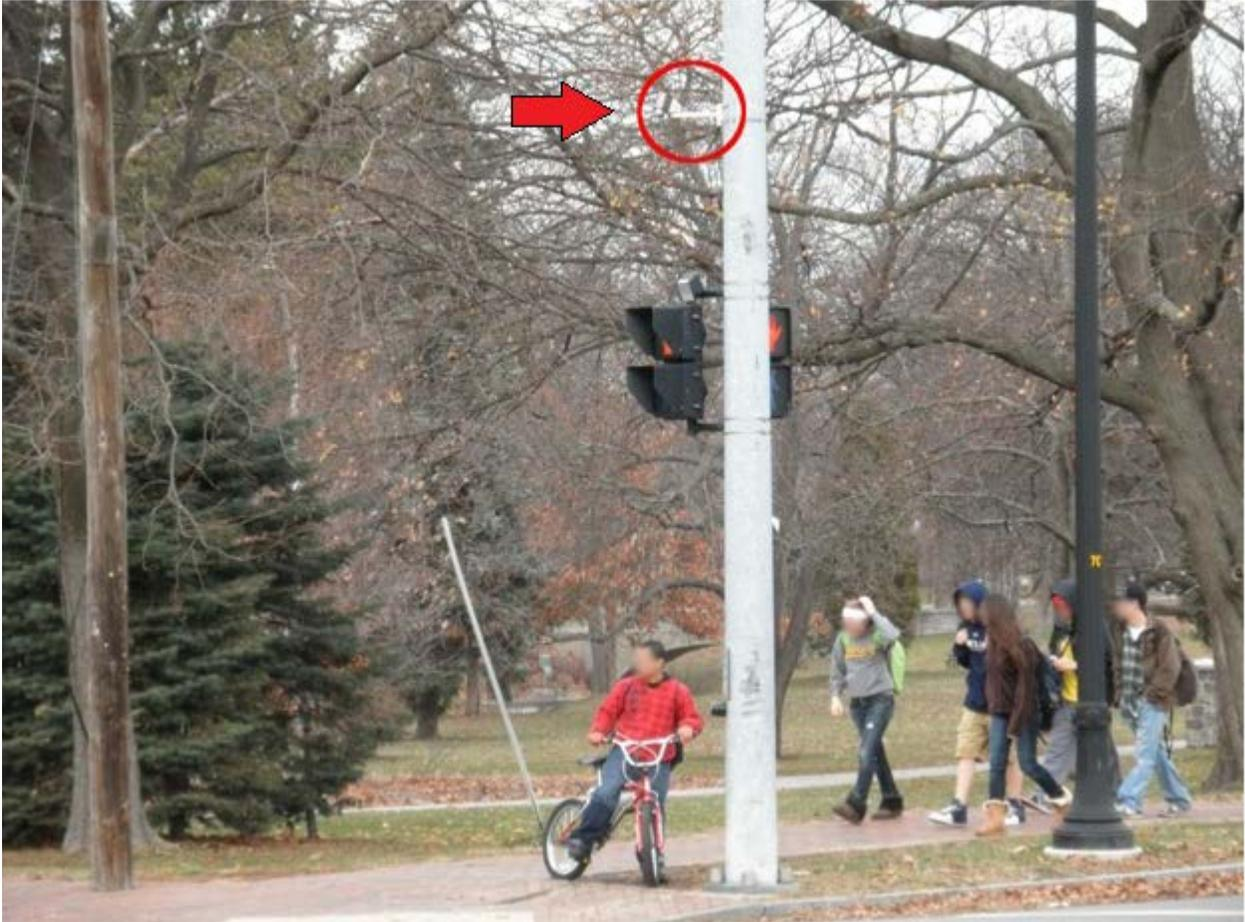
**Figure 25. Photo. Operational stereo pedestrian detection system at Deering Avenue and Park Avenue in Portland, ME.**
