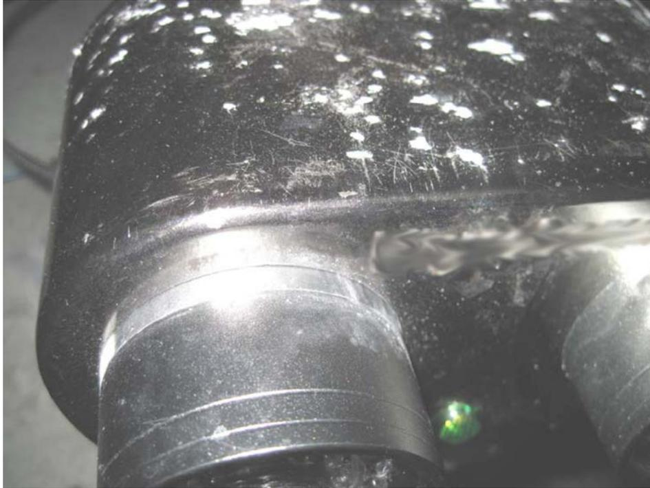
Photograph 5: Loose Lens on Sample 1 Post Vertical Axis
