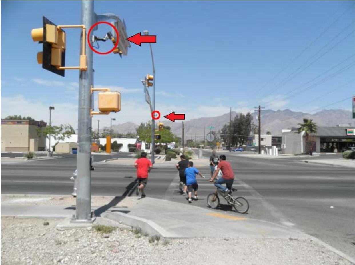
**Figure 19. Photo. Operational stereo pedestrian detection system on the west side of the intersection at East Grant Road and North Palo Verde Boulevard in Tucson, AZ.**
