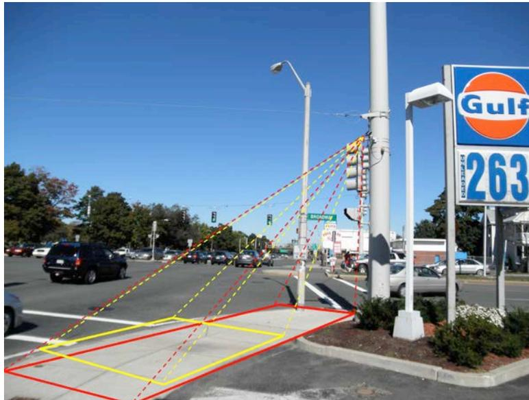
**Figure 4. Photo. Two-zone detection architecture for locator triggering and pushbutton actuation.**
