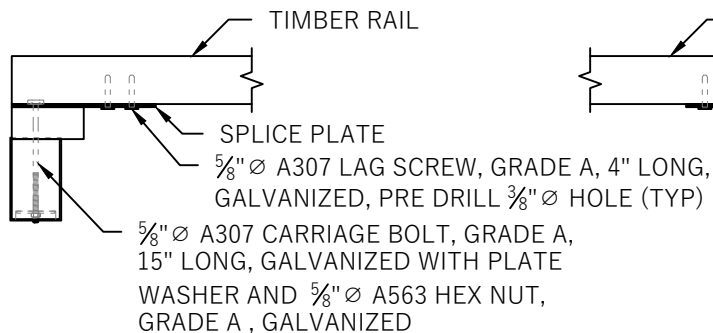
POST / RAIL CONNECTION AT POST 1
