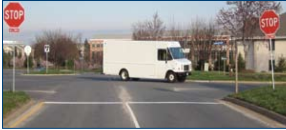
Additional (left and right side of street) and larger (30-inch) stop signs with stop bars.
