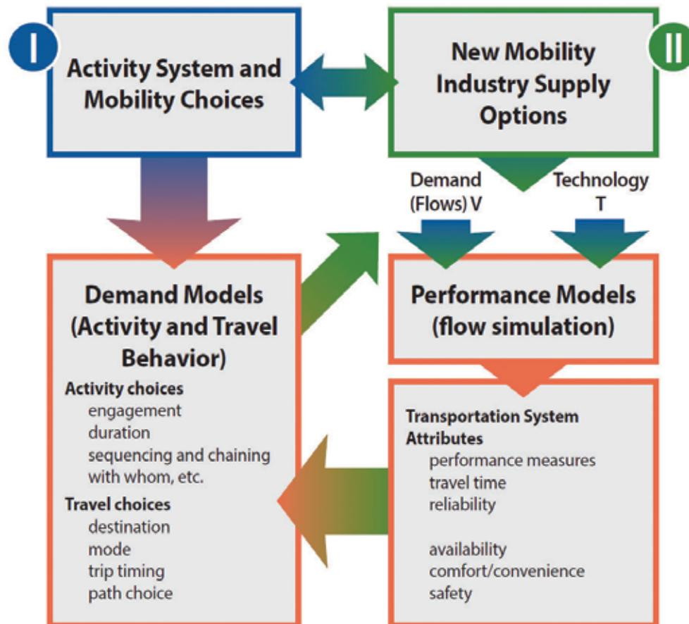
**Figure 1.** Methodological framework for network- and system-level assessment of CAV impacts. (Source: FHWA).<sup>1</sup>
