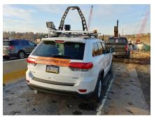
Vehicles used for automated speed enforcement in Pennsylvania work zones featuring enforcement signage. (Source: Pennsylvania DOT)
