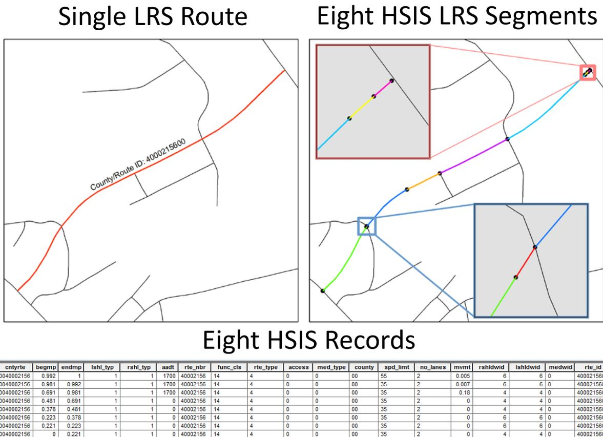
Figure 2: GIS processing, single linear reference system route, supported by eight underlying records.
