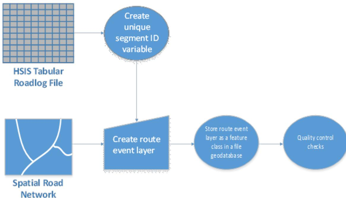
**Figure 1: General process for mapping HSIS road log data to spatial network.**
