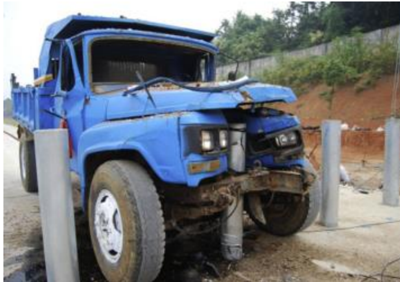
Figure 8. Photo. Anti-ram bollard impact field test.
