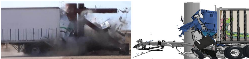
(a) Trailer impact on pier during field testing. (b) Trailer impact on pier in LS-DYNA.
