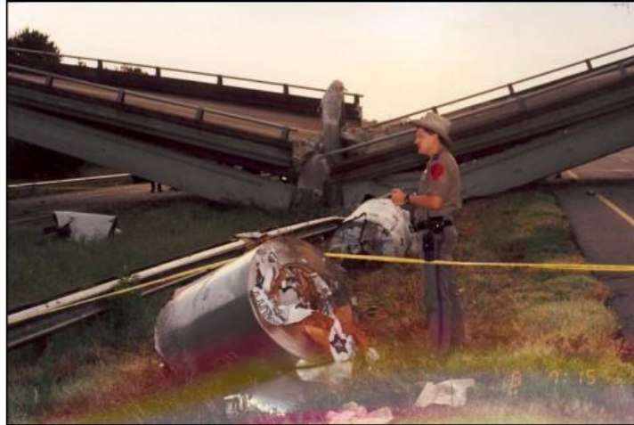
Figure 4. Photo. Truck impact on FM 2110 bridge over IH-30, Texarkana, Texas on August 8, 1994.
