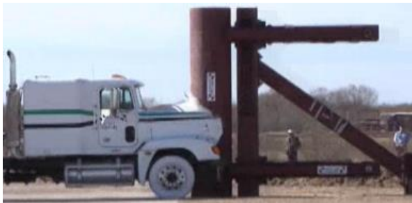
(a) Engine impact on pier during field testing. (b) Engine impact on pier in LS-DYNA.
