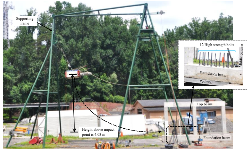
Figure 56. Photo. Setup of field test.
