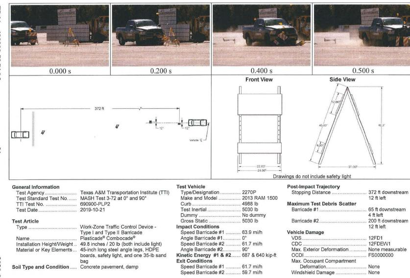
Figure 6.7. Summary of Results for MASH Test 3-72 at 0° and 90° on Plasticade® Combocade®.
