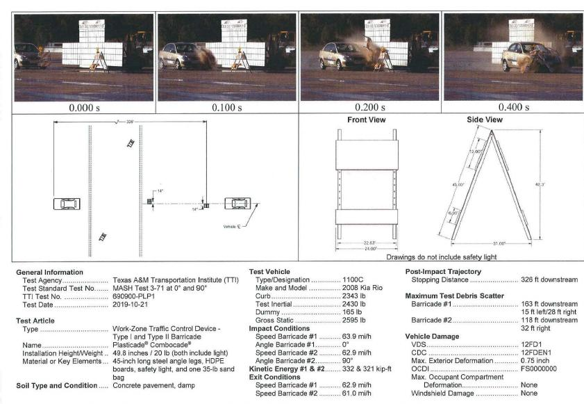
Figure 5.7. Summary of Results for MASH Test 3-71 at 0° and 90° on Plasticade® Combocade®.
