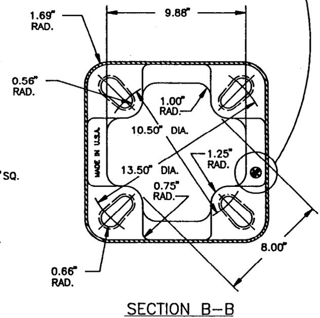
MIG 4043 WIRE 0.25 P WITH APPROXIMATELY 5" OF WELD ON EACH OF THE (4) INTERNAL CORNERS
