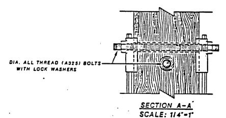
Figure 9. AD-IV Hinge (Upper Connection)
