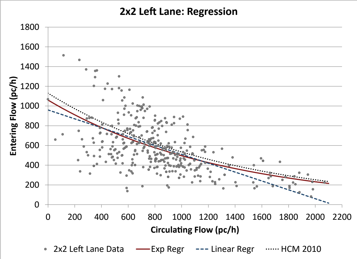
Figure 39. Scatter Plot. Regression models for multilane, 2x2 roundabout sites, left entry lane.
