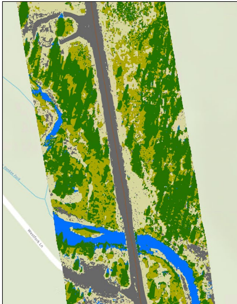
Figure 20. Graphic. Classified NAIP imagery used for roadside object analysis in Idaho.
