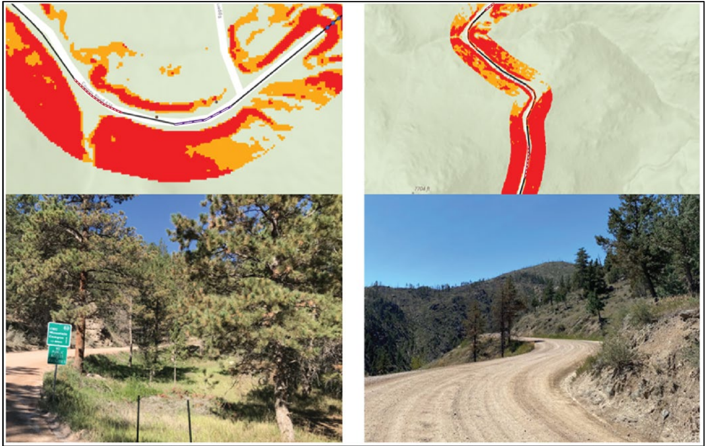
Figure 23. Graphic. Parallel examples of non-traversable slope and roadside hazard in Larimer, CO.
