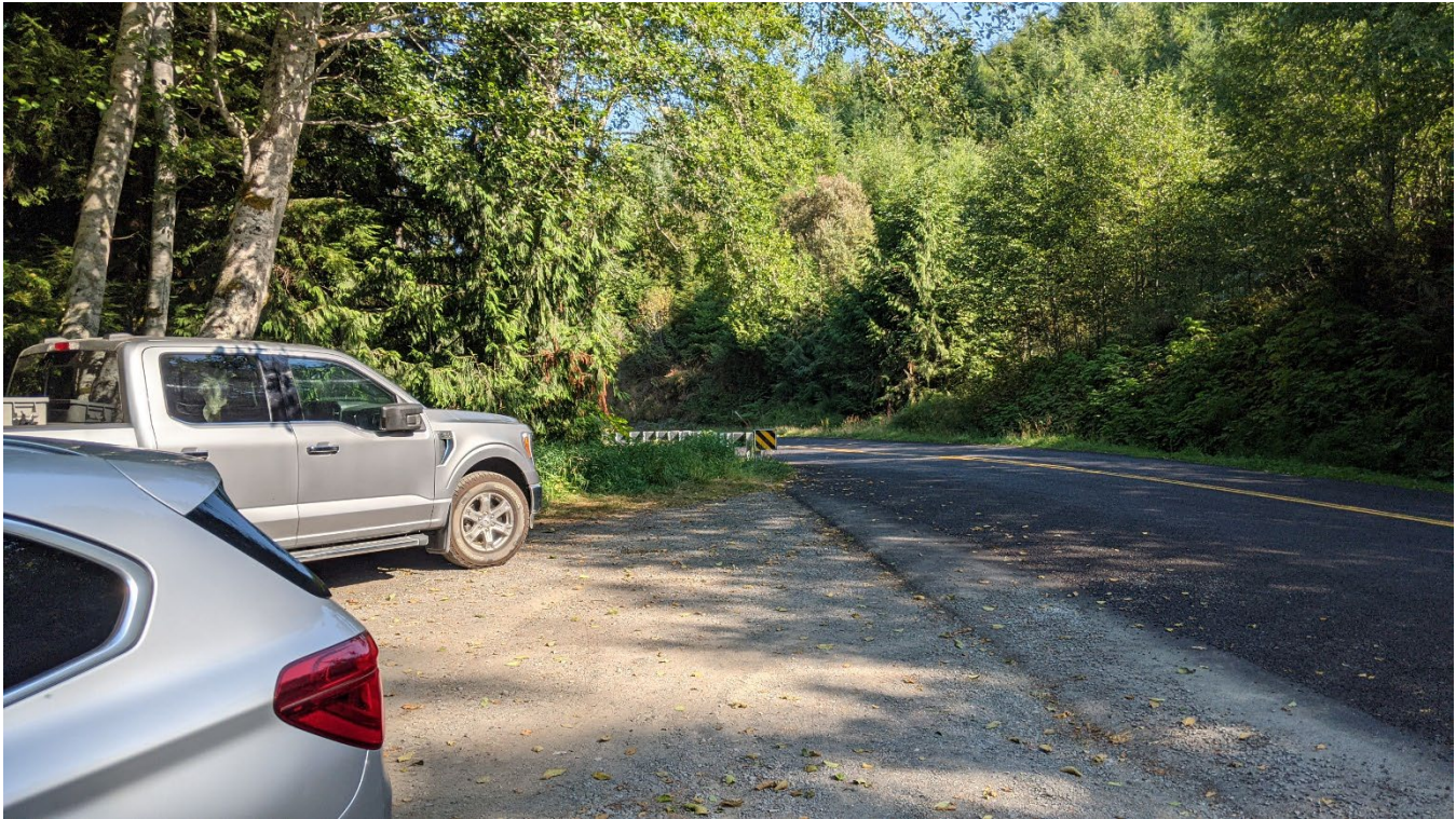
Figure 92. Photograph. Example of parking turnout with sight distance limitations due to curvature.
