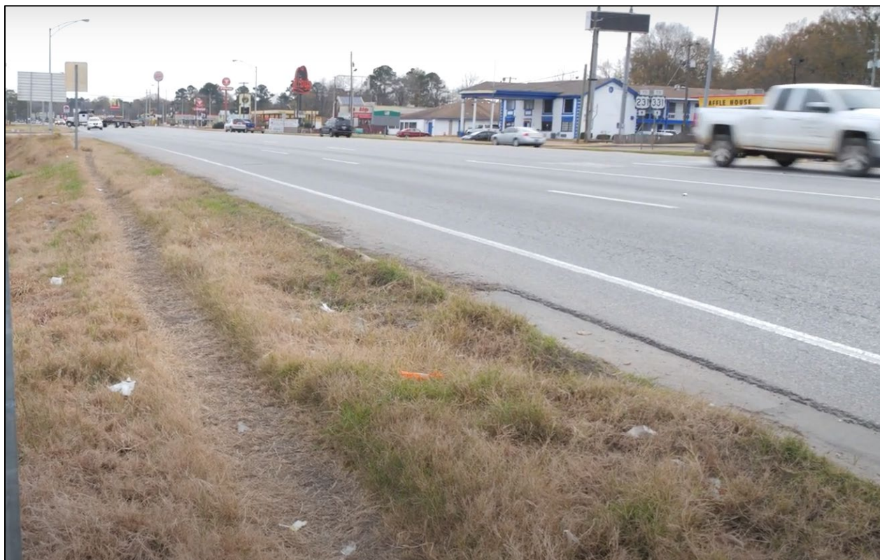
Figure 83. Photograph. Example of an informal desire path created by pedestrians. (63)
