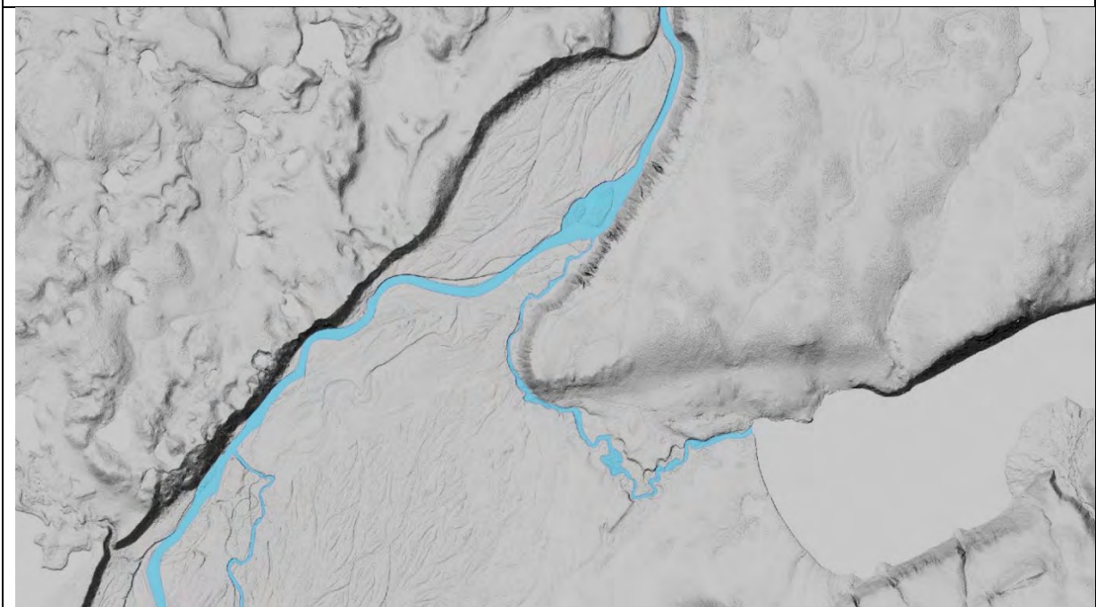
Figure E - 8. LiDAR DEM showing the active channel (outlined in blue) at the outlet of Copper Lake. Note that the active channel does not include the wider floodplain of the Copper River.
