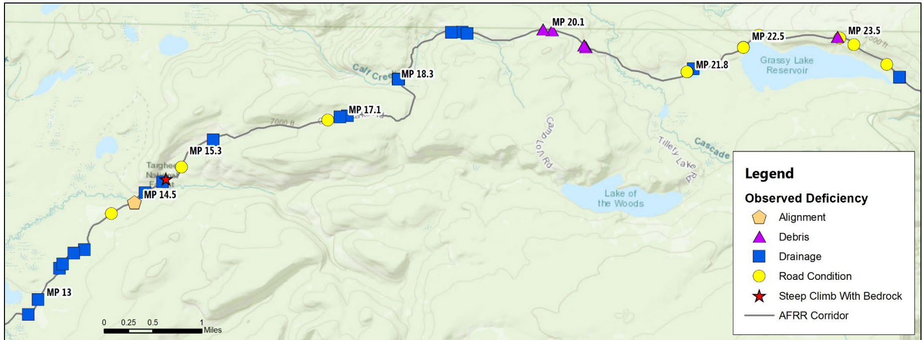
Figure 21: Observed Deficiencies on AFRR Between MP 12.8 and MP 24.5
