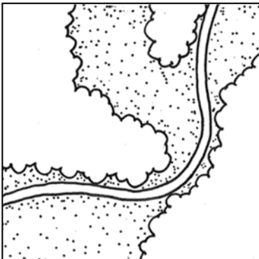
Roadway Design Guidelines DE-4: Consider road geometries for lower speeds, safety and alertness
