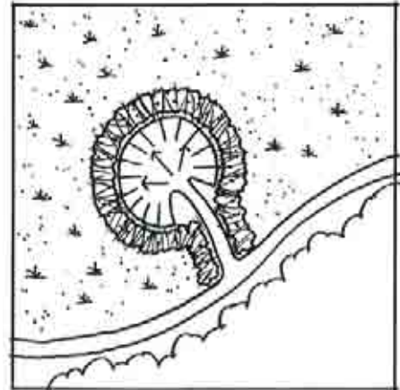
NDS features receive, clean and detain or retain runoff from roadways and other impervious surfaces; they can buffer habitat areas from negative ecological impacts.
