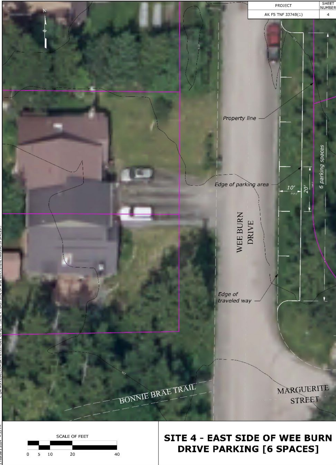
Figure 12. Proposed conceptual site design for Site 4, with on-street parallel parking spaces along the east side of Wee Burn Drive.
