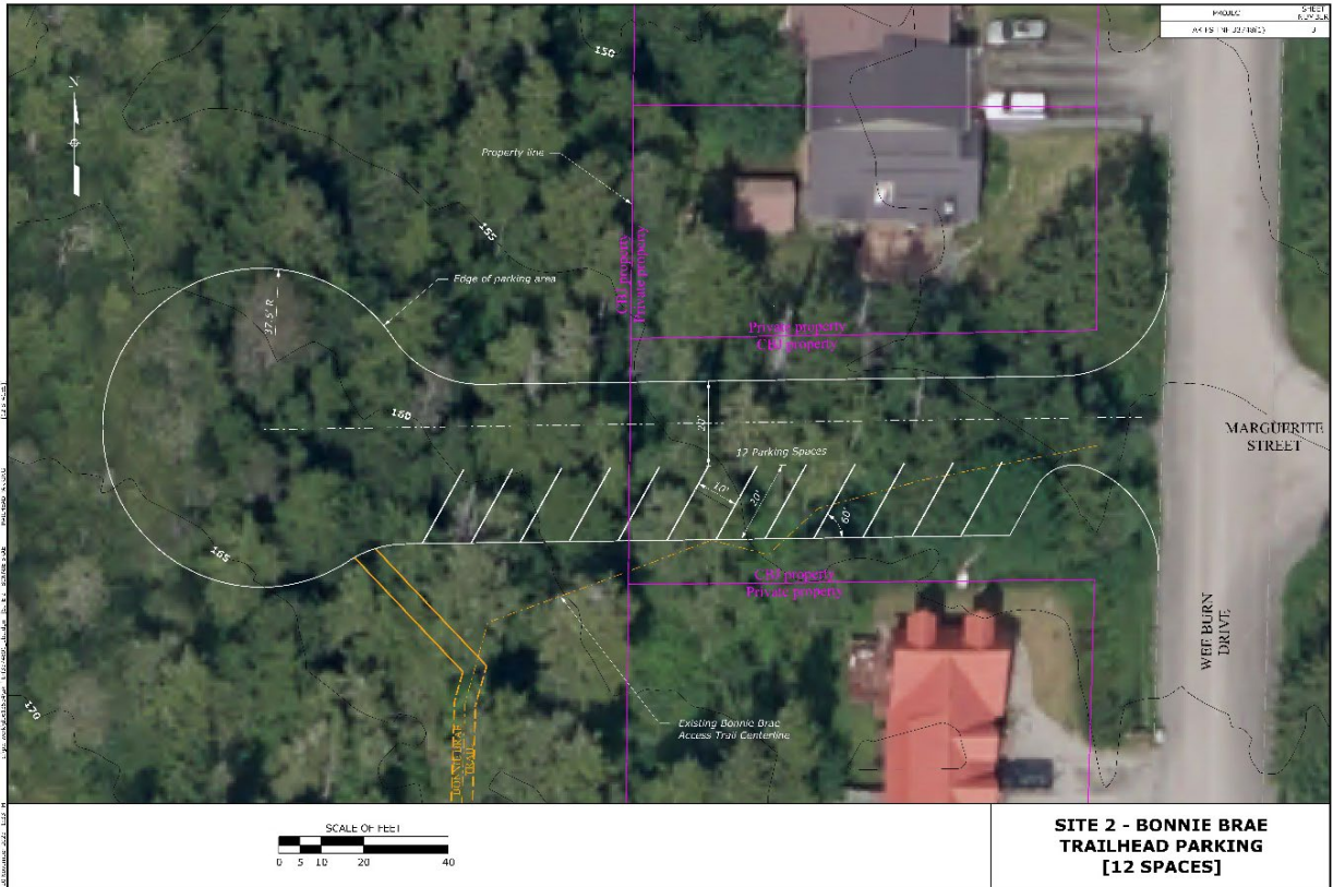
Figure 9. Site 2 at existing Bonnie Brae Access trailhead with up to 12 angled parking spaces along a driveway with turnaround off of Wee Burn Drive
