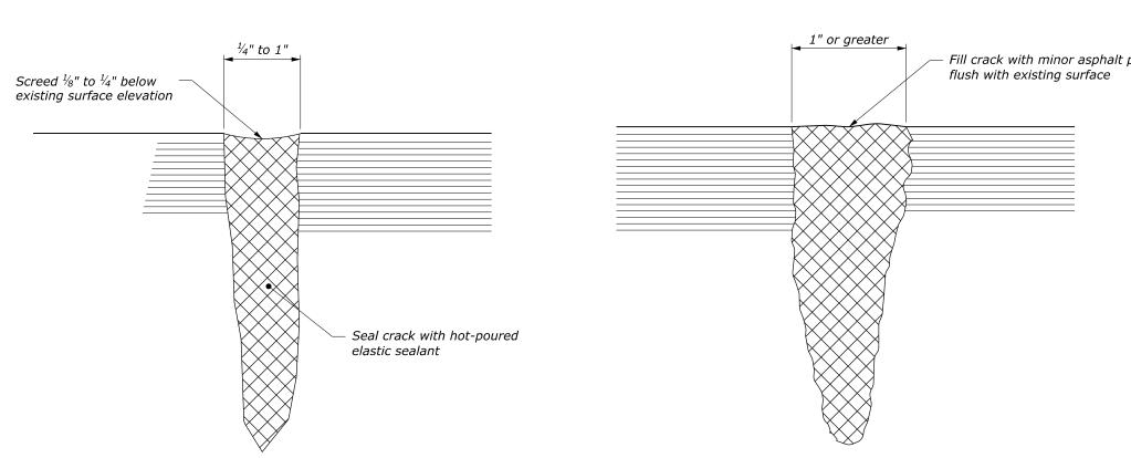
CRACK SEALING DETAILS
