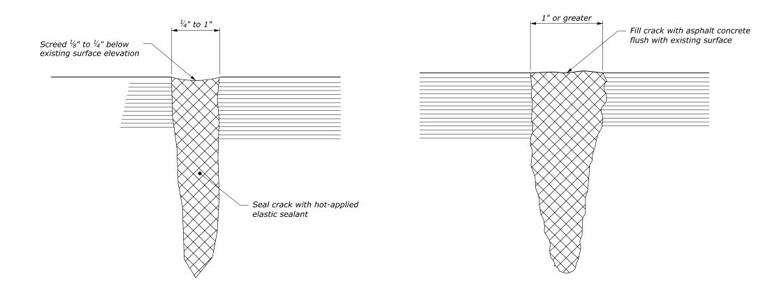
CRACK SEALING DETAILS
