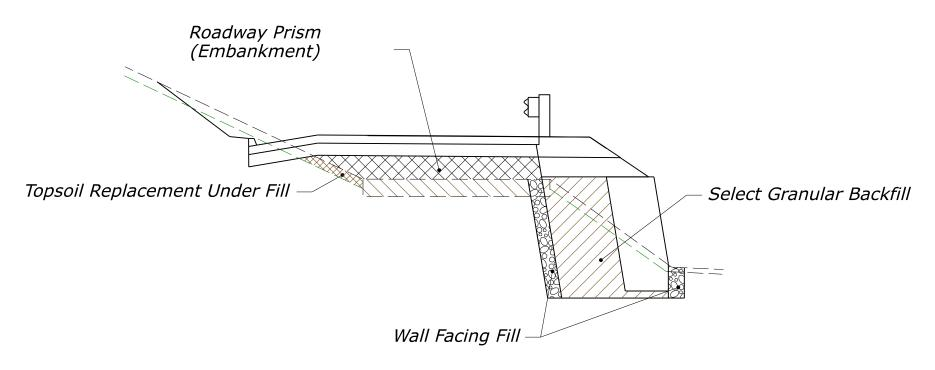
ROADWAY EMBANKMENT GABION FACED MSE
