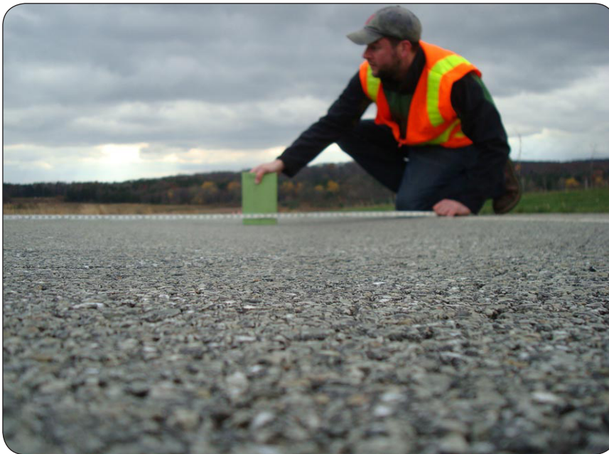
Sean O'Brien, FLH Pavement Engineer capturing field measurements of asphalt pavement rut depth Flight 93 National Memorial Ring Road, Pennsylvania
