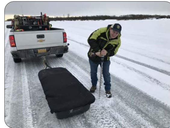
Ground penetrating radar sled used to monitor ice road thickness, drill in operation to measure thickness of the ice. Drilling through ice roads to measure their thickness is now only required occasionally to calibrate the ground penetrating radar sled.
